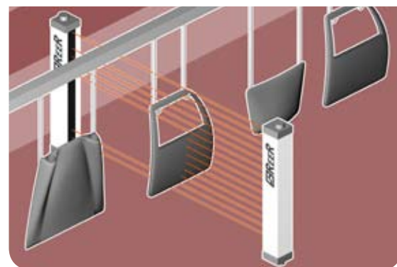
Detection of position and profile of pieces in automatic painting systems
